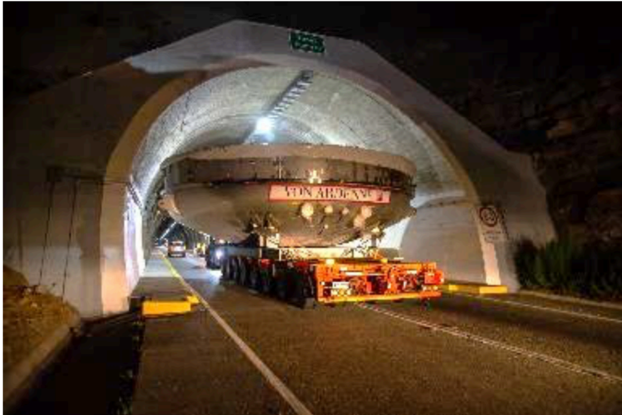
Optical Coating Chamber in transit to the summit – Puclaro Tunnel
